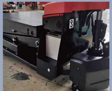
The batteries can be removed conveniently, for easier maintenance and disassembly
