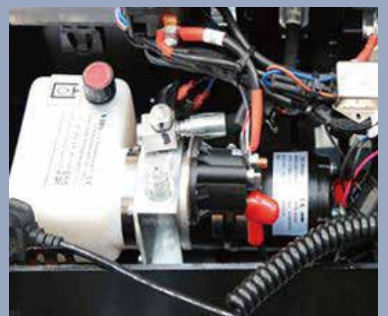
Integrated hydraulic unit, compact structure, less space
